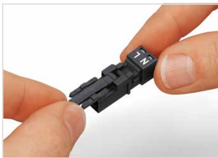
All connectors for mounted installations (snap-in versions, pluggable PCB connectors, distribution connectors) are factory-equipped with locking levers to ensure plugs and sockets are securely locked. Additional locking levers are only required for "flying leads" (plug/socket).
