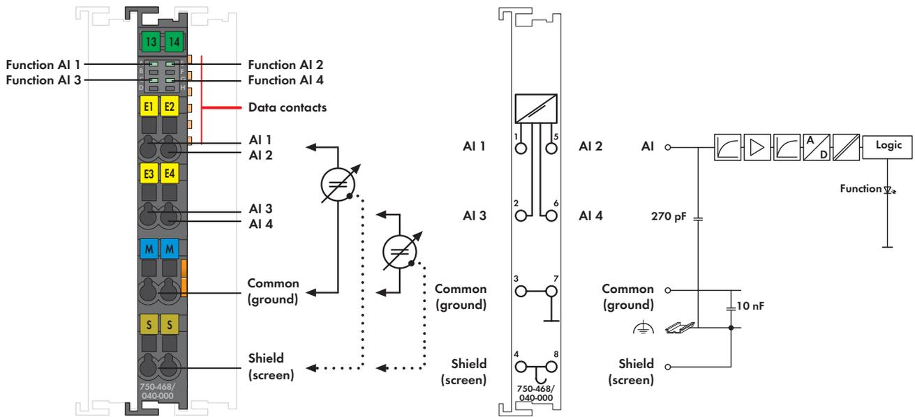
The analog input module processes standard 0-10 V signals. The input signal is electrically isolated and transmitted with a resolution of 12 bits. The internal system supply powers the module. The input channels of the module have a common ground potential. The shield (screen) is directly connected to the DIN rail.
