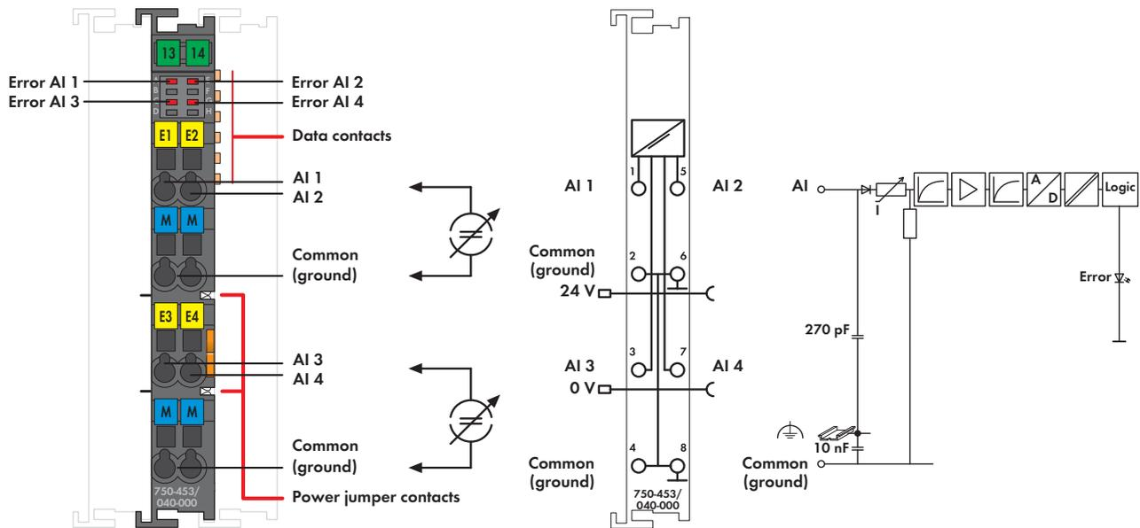
The analog input module processes standard 4-20 mA signals.
