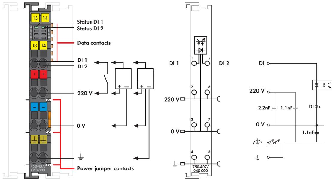
The digital input module receives control signals from digital field devices (e.g., sensors). The module is a 4-conductor device allowing direct connection of sensors with ground contact. Each input module has a 3.0 ms noise-rejection filter. Field and system levels are electrically isolated. The field power must be reapplied after every 7 modules.
