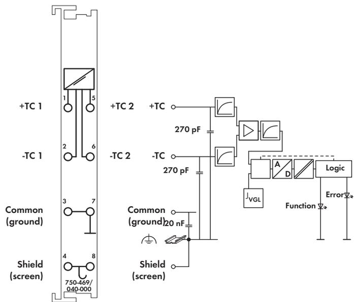
This input module directly connects to two thermocouples. Internal electrical isolation allows operation of grounded sensors. The bus module linearizes the entire temperature range. Cold junction compensation mitigates the clamping unit offset voltage over the 0–55 °C operating range. A line break is indicated by a red LED. A green LED indicates readiness for operation and error-free communication with the bus coupler. The shield (screen) is directly connected to the DIN rail.
