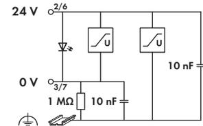
The WAGO-I/O-SYSTEM 750 XTR can also be used in shipbuilding applications and onshore/offshore installations (e.g., platforms, loading facilities). This is possible via certification under the standards of leading agencies such as Germanischer Lloyd and Lloyds Register. Proper system operation is ensured (certified) by using this overvoltage protection module. This also applies to XTR I/O modules used in substations and/or telecontrol systems.
