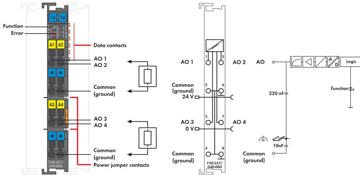
This analog output module generates standard  $\pm 10$  V or 0-10 V signals. The output signal is electrically isolated and transmitted with a resolution of 12 bits. The internal system supply powers the module. The output channels of the module have a common ground potential.
