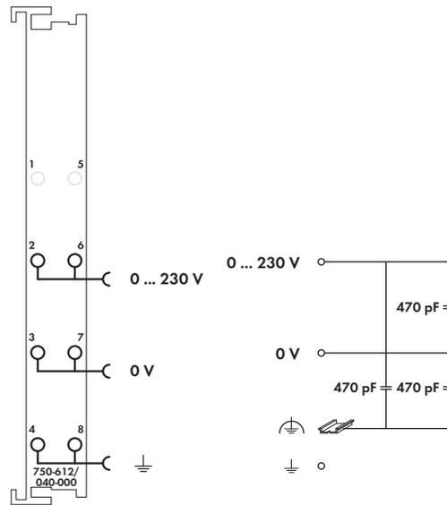
This supply module provides the I/O modules with the corresponding supply potential. Maximum available supply current to all connected modules is 10 A. When configuring the system, it must be ensured that this total current is not exceeded. Should higher currents be necessary, an intermediate supply module must be added to the assembly.
