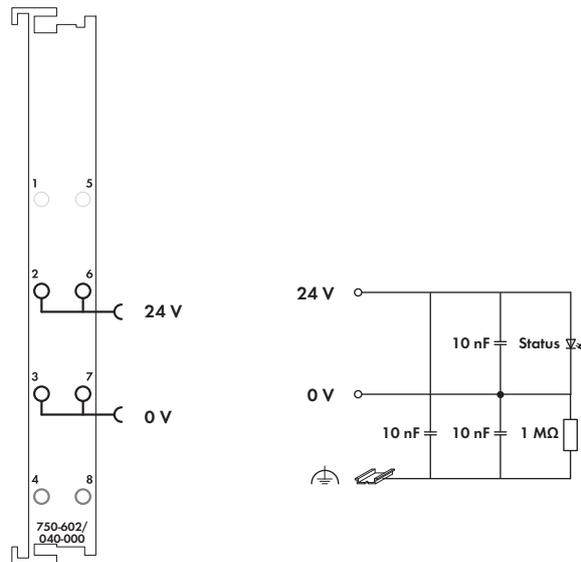
This supply module provides the I/O modules with the corresponding supply potential.
