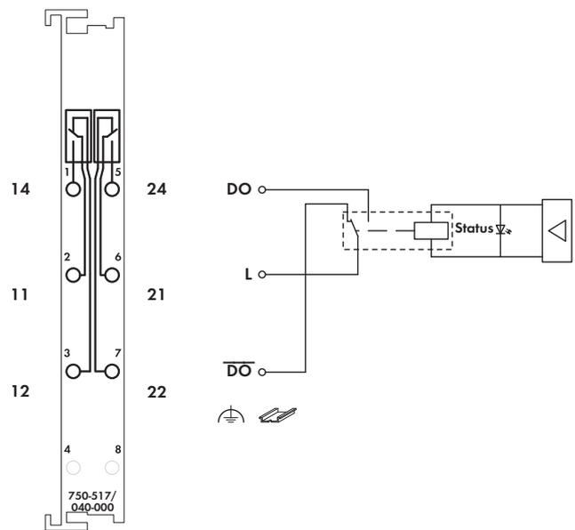
This digital output module transmits control signals from the automation device to the connected actuators. The internal system voltage triggers the relay. The NO contacts are electrically isolated. The switched status of the relay is shown by a LED.
