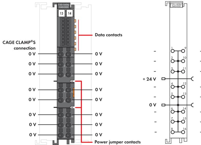
This field-side connection module is used in combination with the 16-channel 750-1504 Output Module (also suitable for 8-channel output modules with a single conductor connection) for providing the 0 V potential to the outputs. This eliminates the need for additional terminal blocks.
