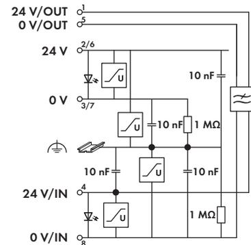
The WAGO I/O-SYSTEM 750 XTR can also be used in shipbuilding applications and onshore/offshore installations (e.g., platforms, loading facilities). This is possible via certification under the standards of leading agencies such as Germanischer Lloyd and Lloyds Register. Proper system operation is ensured (certified) by using this overvoltage protection module. This also applies to XTR I/O modules used in substations and/or telecontrol systems.
