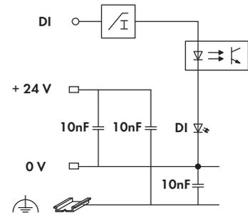
This 2-wire digital input module provides 8 channels at a width of just 12 mm. It receives binary control signals from digital field devices (e.g., sensors, encoders, switches or proximity switches). The module features CAGE CLAMP<sup>®</sup>S connections providing push-in termination of solid conductors. Each input channel has a noise-rejection RC filter with 3.0 ms time constant. A green LED indicates the switched status of each channel. Field and system levels are electrically isolated.
