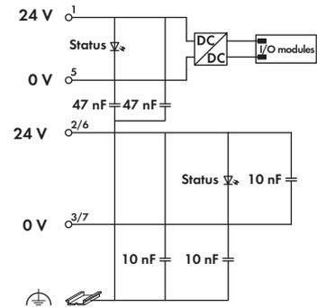
This internal system supply module increases the current supply for the internal system by 2 A. If the internal current consumption of all modules is higher than 2 A, an additional supply module must be added. The module also supplies field side power to the adjoining modules via the power jumper contacts.
