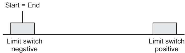
Fig. 3.11.1-14: Referencing to limit switch starting in negative direction from negative limit switch g067x41e
